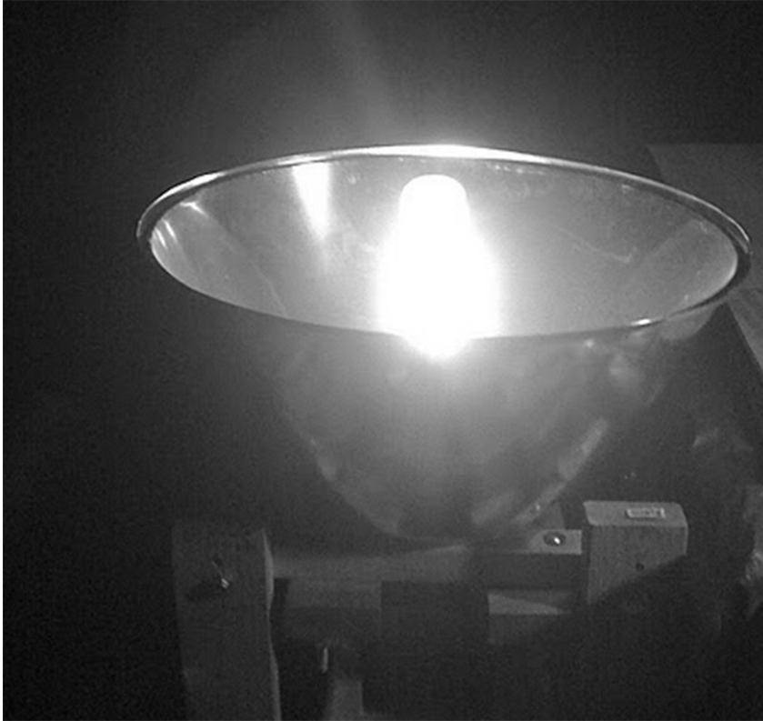
Figure 3 – A 1000 watt high pressure sodium light with the aluminum reflector.
