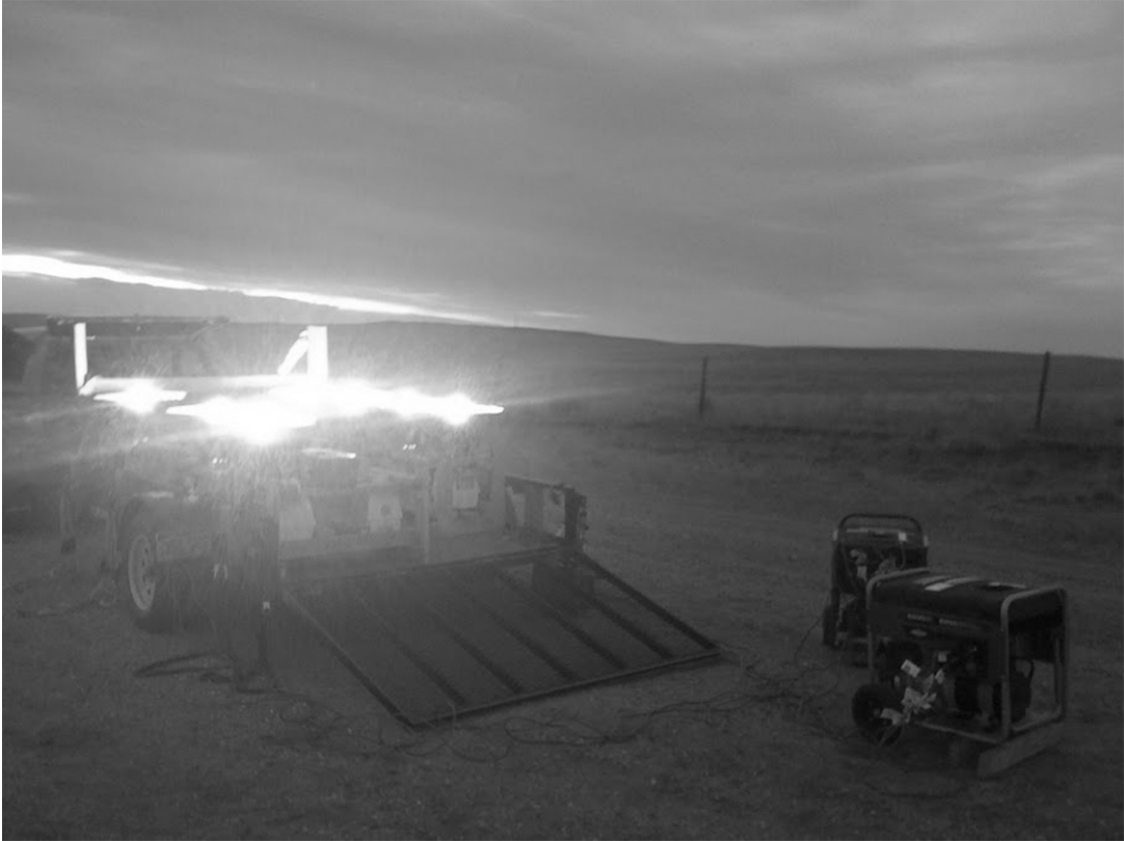
Figure 4 – Seven (1000 watt) high pressure sodium lights in the utility trailer and the two generators used to power the lights in the field.
